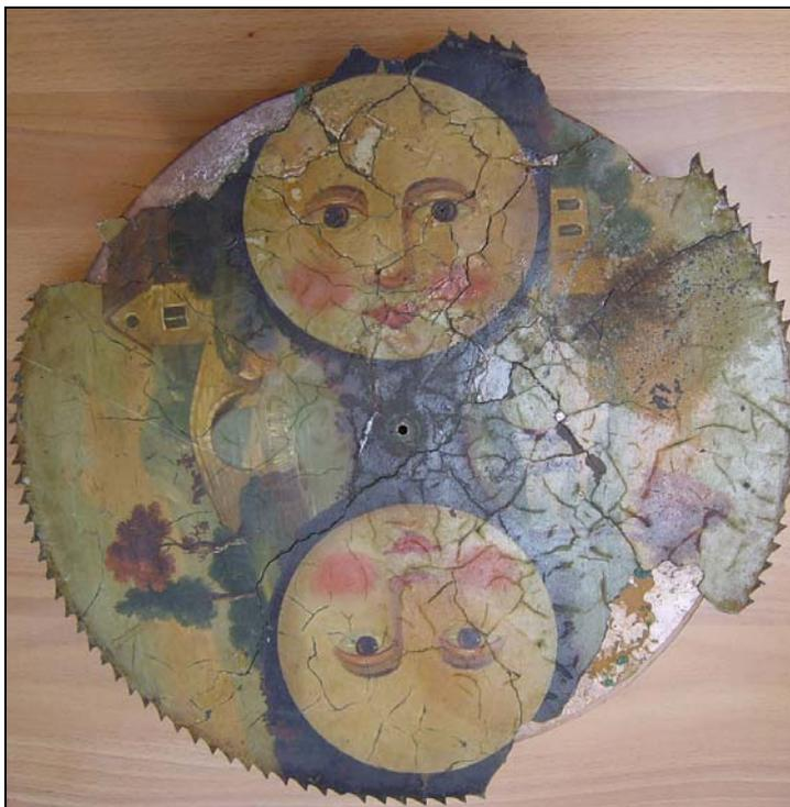
The original dial, showing the severity of the brass fatigue fractures. These discs were often made from poor quality off cuts of flat cast brass.
